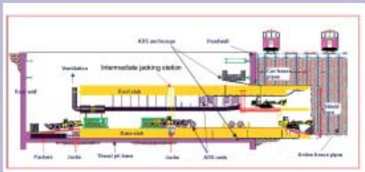
Figure 6 Jacked tunnel – long section showing overall system
