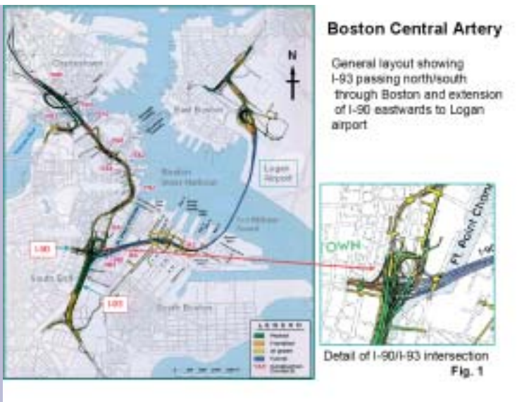
Figure 1 Boston Central Artery: General layout showing I-93 passing north/south through Boston and extension of I-90 eastwards to Logan airport
