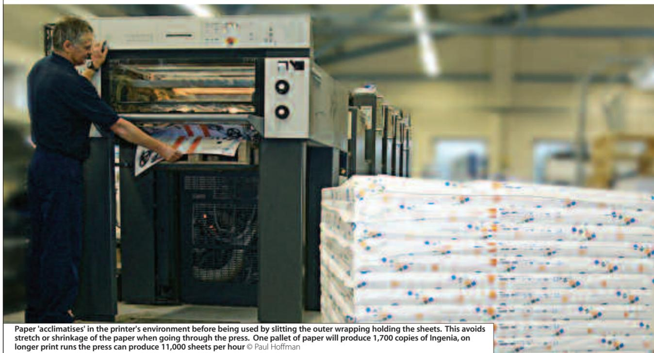
Paper 'acclimatises' in the printer's environment before being used by slitting the outer wrapping holding the sheets. This avoids stretch or shrinkage of the paper when going through the press. One pallet of paper will produce 1,700 copies of *Ingenia*, on longer print runs the press can produce 11,000 sheets per hour © Paul Hoffman
