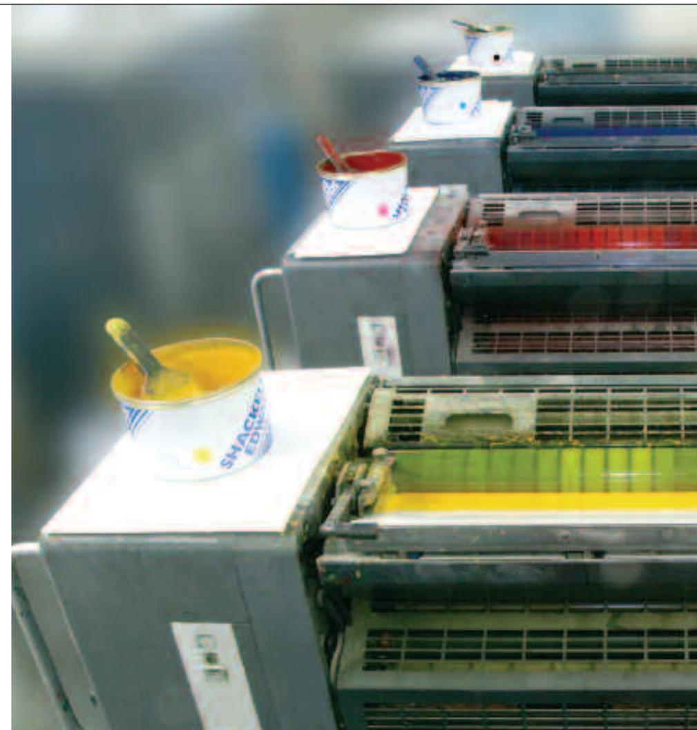
Four ink towers on top of the five colour press. Ink (yellow, magenta, cyan and black) is poured into the open ducts and then distributed evenly through 24 rollers within the towers arriving on each plate as a very fine film © Paul Hoffman
