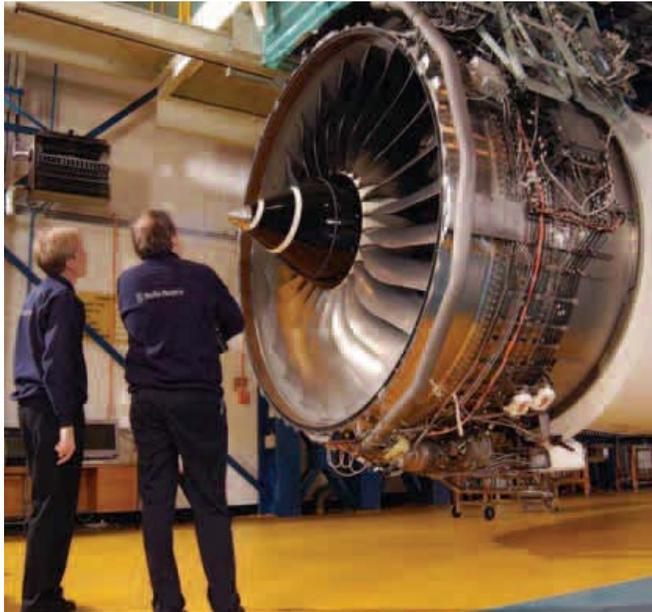
The Trent 900 engine powers the Airbus A380 airliner © Rolls-Royce plc
