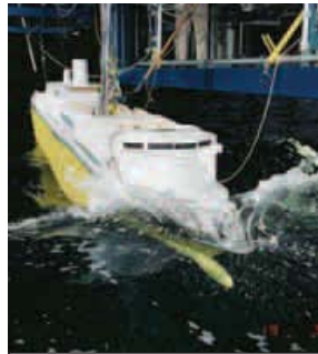
The original models for the Queen Mary 2 had four pods and a rudder. Model-testing showed that the size of the rudder needed to influence and start steering the ship was so large, and introduced such a high drag, that we felt this could be better achieved by just using pods © Chantiers de l'Atlantique
