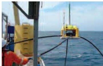
Deployment of an OHM long dipole receiver
