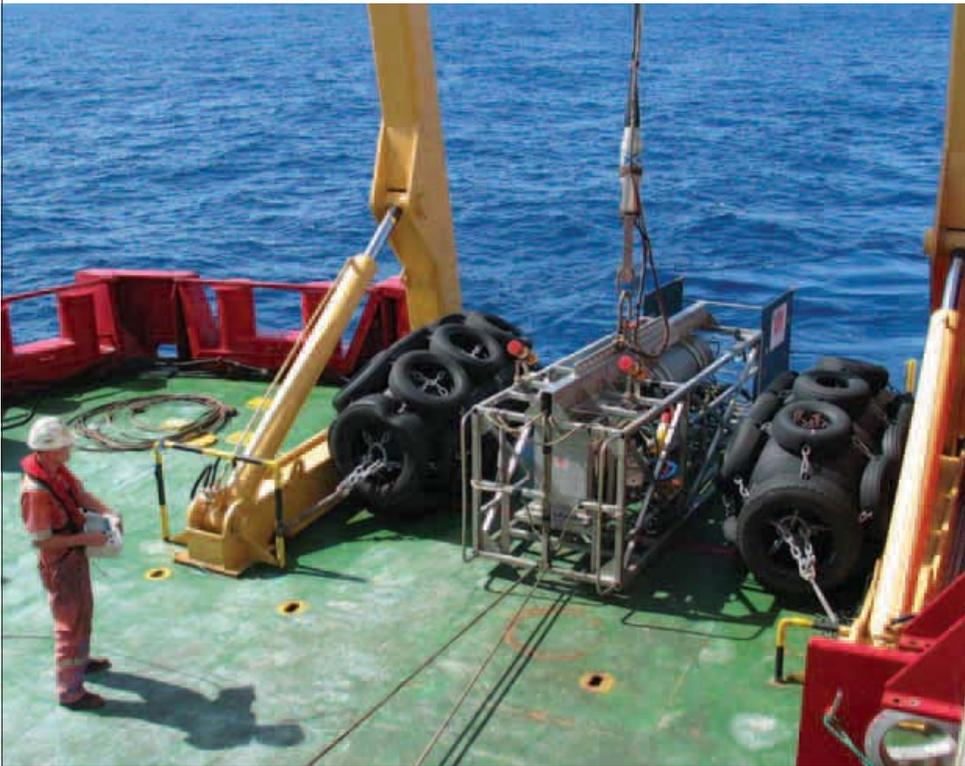
A DASI CSEM transmitter on a board a survey vessel. This electromagnetic transmitter uses a horizontal electrical dipole to generate an electromagnetic signal about 30 metres from the seafloor. Much of the development in refining CSEM for application to oil and gas exploration has focused on increasing both output strength and phase stability of the source waveform, which are critical for successful detection of resistive layers in a strongly conductive medium © Offshore Hydrocarbon Mapping
