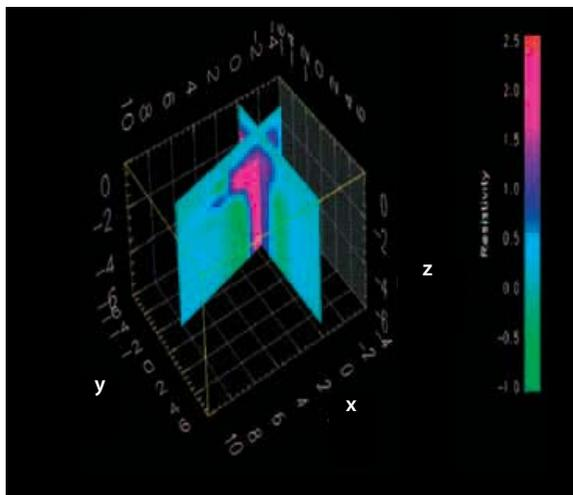
CSEM data can be used to give a cross section of resistivity distribution in the sub-surface. The presence of potentially hydrocarbon-bearing layers can then be assessed by studying vertical and horizontal resistivity variations © Offshore Hydrocarbon Mapping
