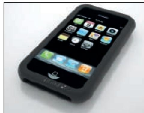
The d3o™ shock-absorbing material is able to be moulded into a variety of shapes, such as a protective outer band for the Apple iPhone © TECH|21
