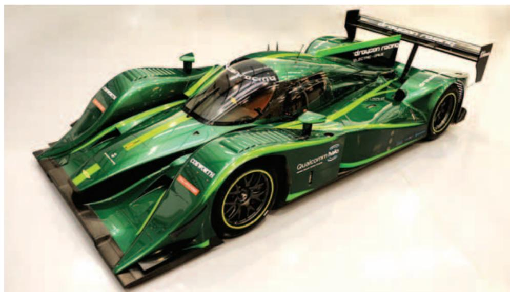
The Lola-Drayson B12/69EV pictured at the Drayson's Kidlington HQ. It is the fastest fully electric racing car. It has a 640kW electric drive, recyclable body panels and wireless charging. When it takes to the track, with a top speed of 200mph it will be one of the most advanced zero-emission competition cars on the circuit
