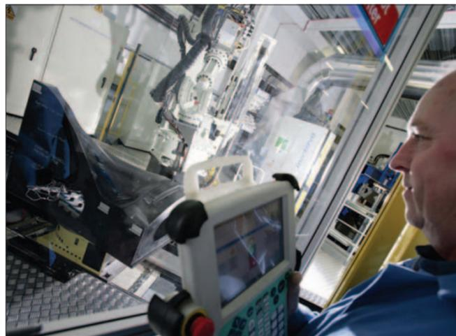
A joint initiative by GKN and Rolls-Royce, CTAL aims to leapfrog the manually-intensive production method of producing carbon composites. They have developed an automated process capable of significantly faster production rates. Here, an engineer is supervising the lamination of hundreds of layers of pre-impregnated fibres to produce considerably lighter fan blades © Rolls-Royce
