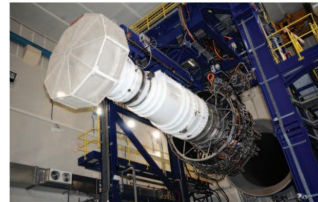
The Environmentally Friendly Engine demonstrator is a heavily modified Trent 1000 with the fan blades removed. Most of the engineering design and analysis on the project was carried out at Rolls-Royce's Derby site, while the assembly and test activity is taking place at Bristol where EFE has a dedicated testbed
