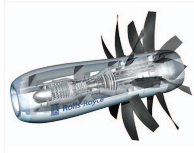
Open rotor concept: open rotor technologies offer the potential for significant reductions in fuel burn and CO<sub>2</sub> emissions relative to turbofan engines of equivalent thrust
