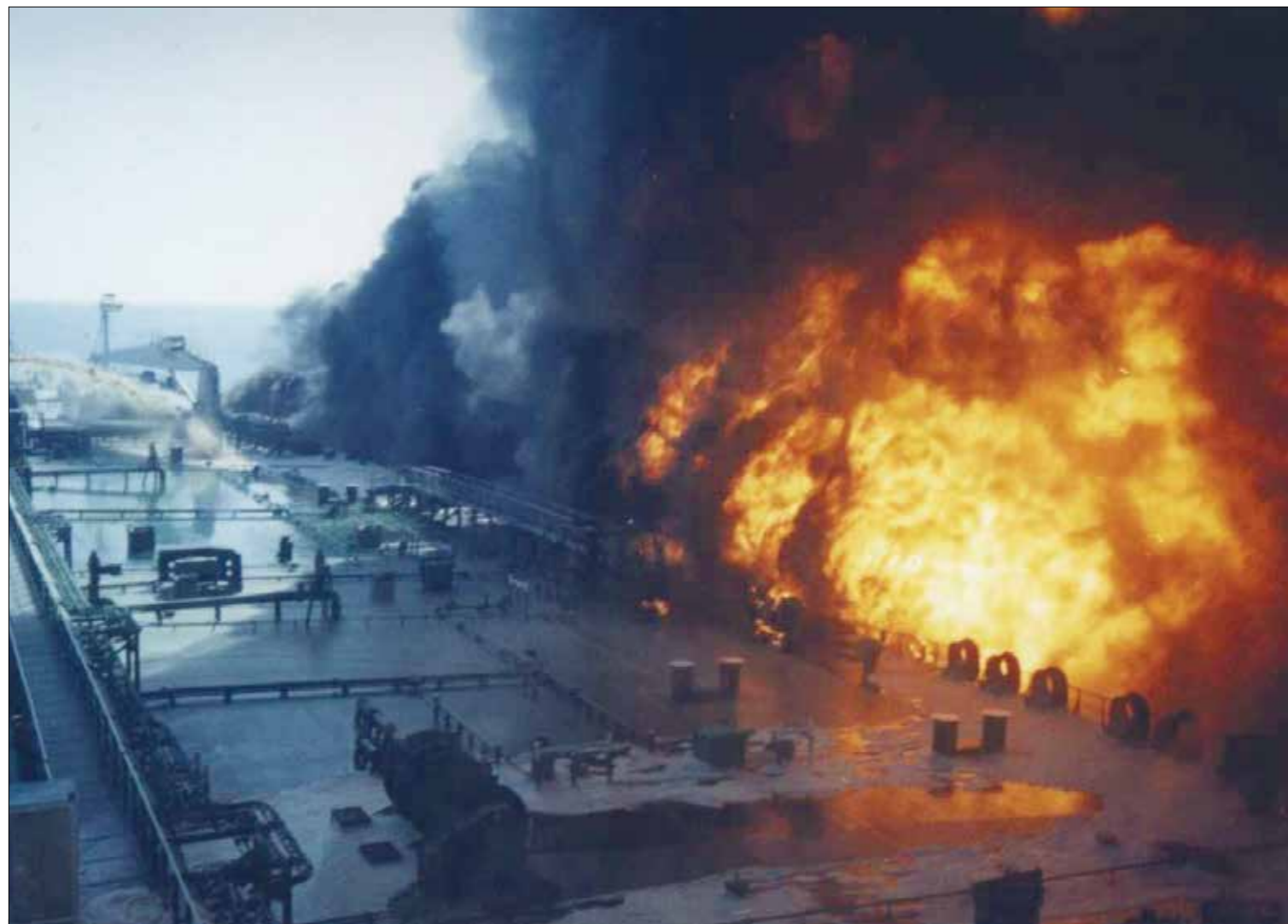
Lloyd's Register's Ship Emergency Response Service (SERS) has had several cases of dealing with fire burning alongside a vessel, as a result of oil spill and ignition following collision, contact with quayside or terrorist attack. Issues with fires include loss in structural strength and changes in loading due to outflow and/or ingress. Heat damage to steel and pool fires can also be extensive and pass along the ship's length
