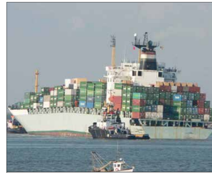
Hull girder failure. This vessel grounded midships following a 6m fall in tide. There was no possibility of remedial action to avoid this outcome. The ship refloated on the next high water with assistance of tugs, but was constrained within a channel due to increased draught caused by the hull deflection. SERS assisted salvors by validating offloading conditions that minimised the bending and shear loads in the hull at the location of the 'bend'. A floating crane was used to move the vessel alongside. The team assisted again with offloading of containers at the quayside and finally with the loading condition suitable for the tow journey to a repair yard © Frans Sanderse
