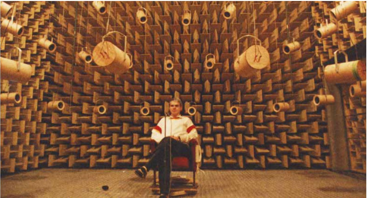
Anechoic chambers are ideal for researching the sound that people hear at home. Pictured is the 3D sound field simulation equipment at the Division of Applied Acoustics, Chalmers University of Technology (c. 1974) © Mendel Kleiner
