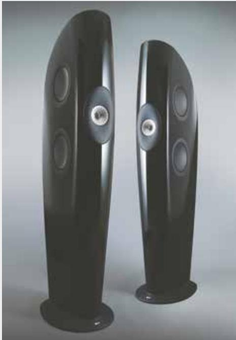
The KEF Blade loudspeaker is designed to have a finely controlled directivity pattern. The high-frequency and mid-frequency drivers are integrated into a combined Uni-Q array on the front of the loudspeaker. The low-frequency drivers are positioned symmetrically around it to mimic the output of an acoustic point source
