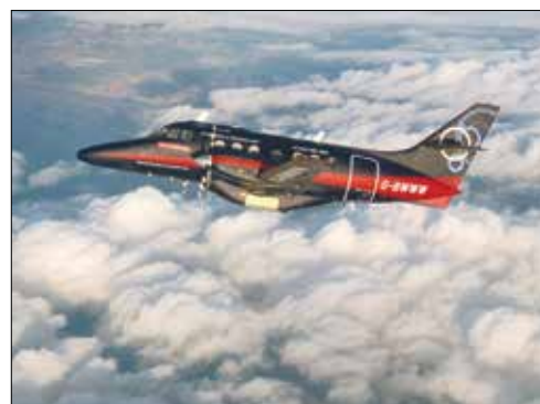
The first flight demonstrating how an unmanned aircraft can operate in all UK airspace took place in April 2013. The adapted Jetstream airliner completed a 500-mile trip from Warton, Lancashire to Inverness, Scotland under the command of a ground-based pilot and control of NATS © BAE Systems
