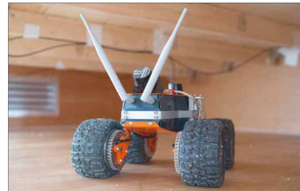
London company, q-bot, develops autonomous tools that enable installers and contractors to access hard-to-reach areas, to survey and understand these environments, building up maps and identifying services that can be provided. They can also apply treatments remotely, such as underfloor insulation © q-bot
