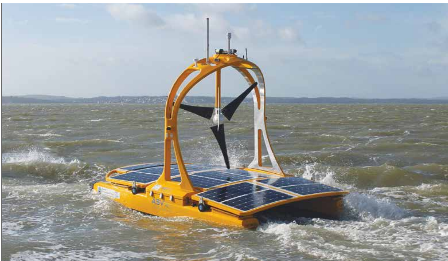
The C-Enduro is one of 50 systems developed by ASV. The autonomous marine vehicle with a self-righting hull can operate for up to three months at a time using a combination of solar, wind and diesel energy. It can be used by oceanographers for a variety of seagoing research missions and for security and defence purposes including chemical detection and anti-submarine warfare © ASV
