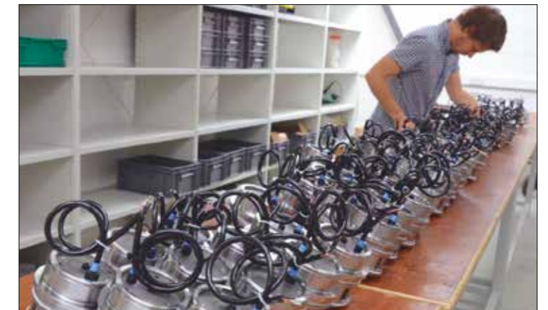
Computer-controlled valves are at the heart of all Artemis hydraulic machines. This batch will be installed in a Digital Displacement® wind-turbine transmission
