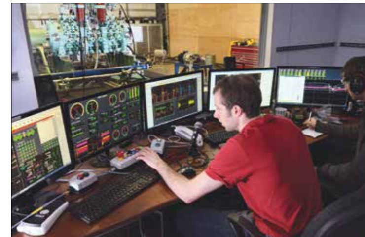
Artemis mechanical engineers testing a 3.5 MW digital displacement motor
