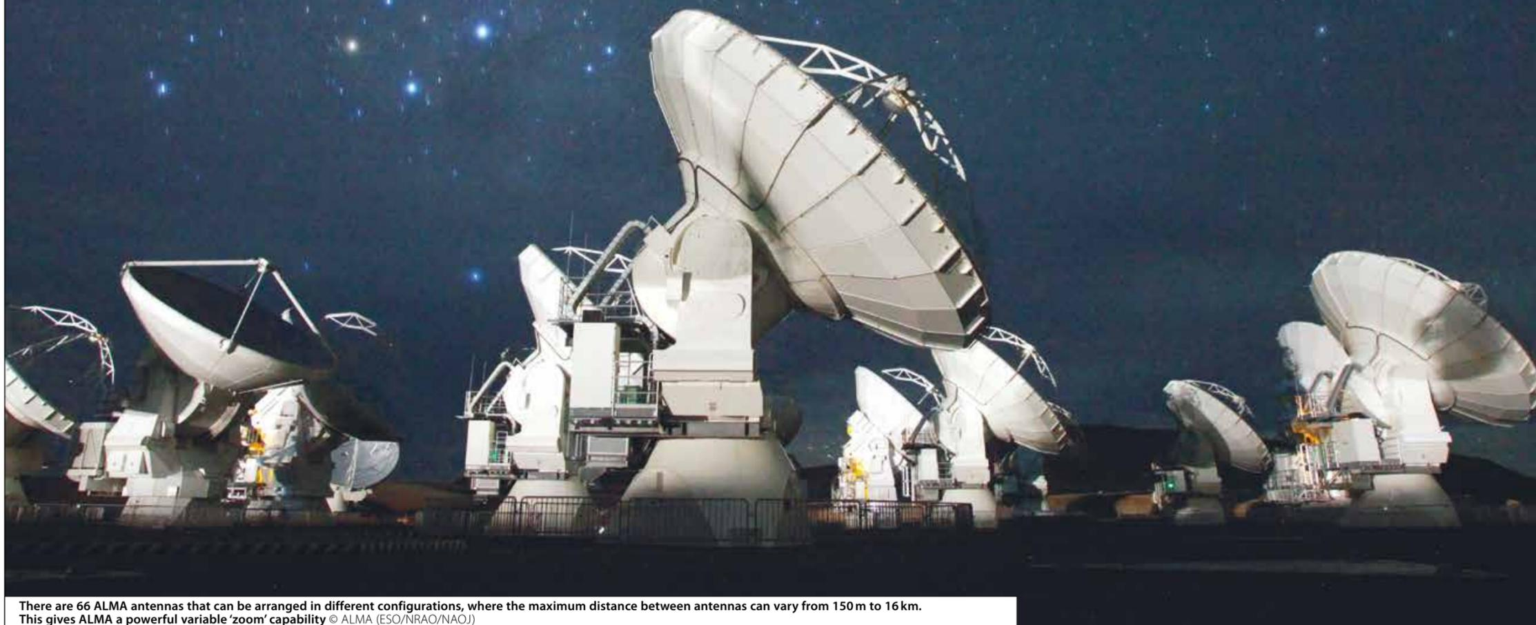
There are 66 ALMA antennas that can be arranged in different configurations, where the maximum distance between antennas can vary from 150 m to 16 km. This gives ALMA a powerful variable 'zoom' capability © ALMA (ESO/NRAO/NAOJ)
