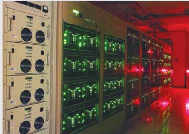
The ALMA Correlator is the world's highest altitude supercomputer. The air is so thin that twice the normal airflow is necessary to cool the machine, which draws some 140 kilowatts of power. Seismic activity is common, so the correlator had to be designed to withstand the vibrations associated with earthquakes © ALMA (ESO/NRAO/NAOJ)
