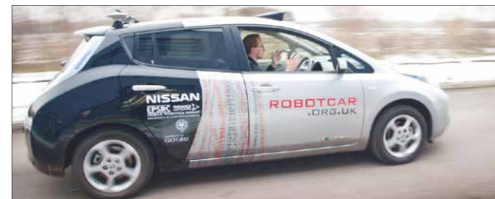
The Mobile Robotics Group's RobotCar is a modified Nissan LEAF electric car. Lasers and cameras provide data for a boot full of electronics that perform the calculations needed to navigate, control speed and to avoid obstacles
