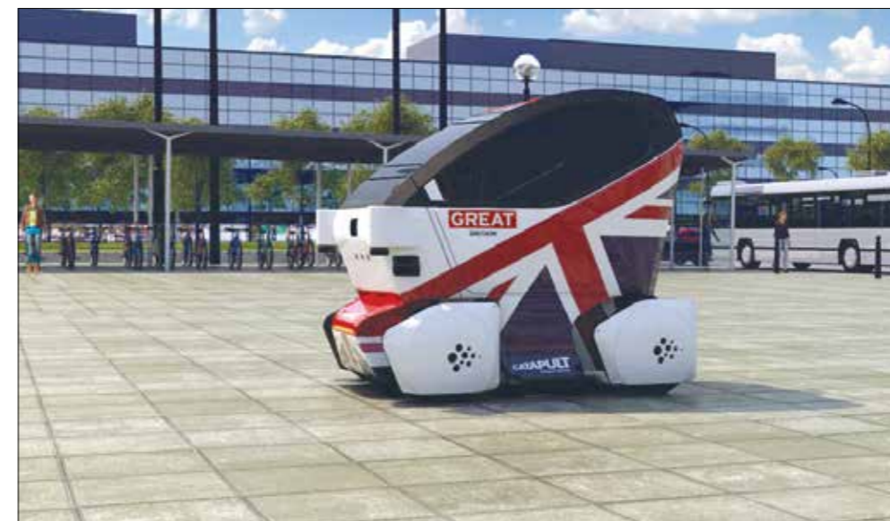
Oxford's Mobile Robotics Group is working with the Transport Systems Catapult and other partners to build autonomous systems into the Lutz pods that will take passengers around Milton Keynes. These systems will eventually do away with the need for a steering wheel or human driver
