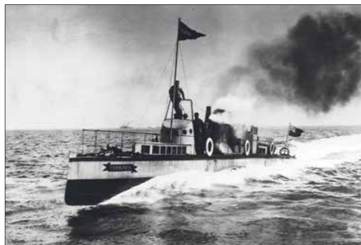
Charles Parsons' steam turbine-powered Turbinia photographed in 1897 by Alfred John West (courtesy Wikipedia BoH)
