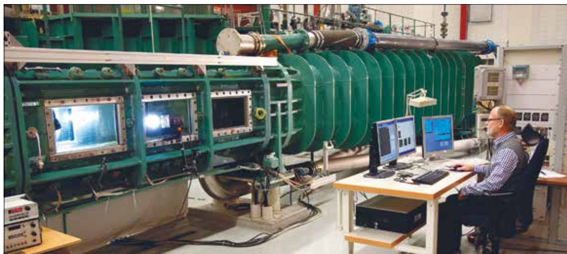
Established in 1971, the Rolls-Royce Hydrodynamic Research Centre in Kristinehamn, Sweden designs and manufactures a range of propulsion systems. These include fixed and controllable pitch propellers, water jets and pods used across a wide range of vessels in the offshore, merchant and naval sectors. It houses two large cavitation tunnels which are used to test a wide range of propeller and impeller designs © Rolls Royce
