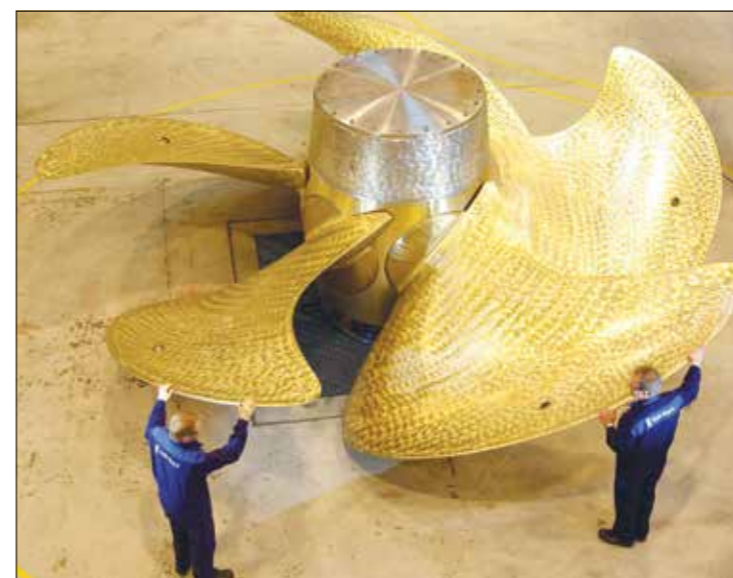
Inspection of one of the QE-class Aircraft carrier propellers prior to delivery from the factory in Kristinehamn, Sweden © Rolls-Royce
