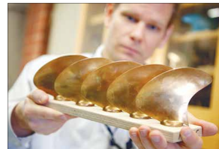
Senior Hydrodynamicist Robert Gustafsson at the Rolls-Royce Hydrodynamics Research Centre holds a five-bladed low-noise propeller design prior to cavitation testing. For optimal efficiency, the multiple blades increase thrust, while they are set in a skewed pattern to reduce noise and vibration © Rolls-Royce
