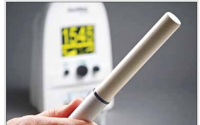
The Sentimag consists of a probe connected to a signal processing unit. The probe is a cylinder 18mm in diameter and 100mm long, which is sheathed during surgery. The signal processing unit has an LCD display that indicates the detected signal with a corresponding audible tone that rises in pitch with the signal intensity. There is also a button to 'balance' the system to set the detected signal to zero © Endomag Ltd
