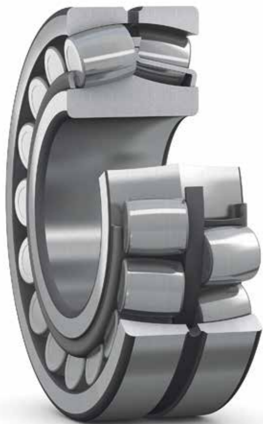
A spherical roller bearing, in which two sets of rollers run on precisely shaped tracks. This design allows very heavy radial loads as well as axial loads to be carried, while tolerating some angular misalignment © SKF
