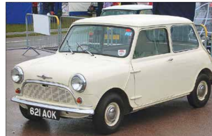
Tribological improvements have significantly contributed to the performance of the Mini. The Morris Mini Minor of the early 1960s with an 850 cc petrol engine had a top speed of 115 km per hour and fuel consumption of 6.6 litres per 100 km. Its successor, the entry-level Mini One with a 1.2 litre petrol engine, can reach 195 km per hour with a fuel consumption (combined cycle) of 4.6 litres per 100 km © DeFacto and Wikimedia Commons
