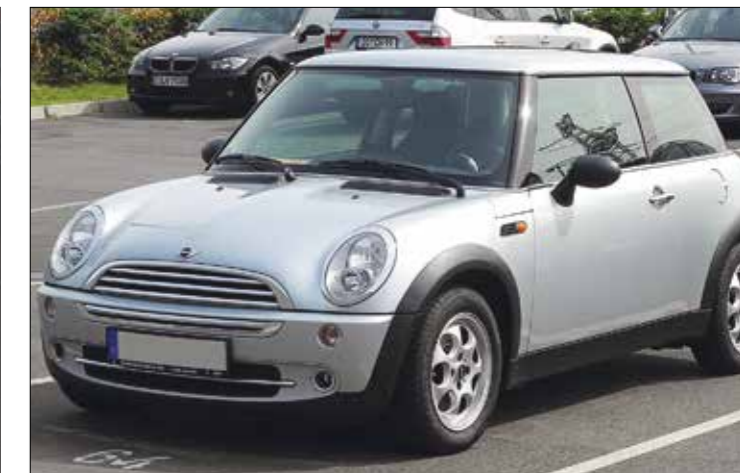
Tribological improvements have significantly contributed to the performance of the Mini. The Morris Mini Minor of the early 1960s with an 850 cc petrol engine had a top speed of 115 km per hour and fuel consumption of 6.6 litres per 100 km. Its successor, the entry-level Mini One with a 1.2 litre petrol engine, can reach 195 km per hour with a fuel consumption (combined cycle) of 4.6 litres per 100 km © DeFacto and Wikimedia Commons
