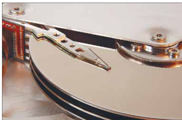
A hard disk head and arm on a platter. The read-write head at the end of a movable supporting arm 'flies' over the surface of the rotating magnetic disk at a height of less than 10 nanometres, supported on a film of air that acts as a lubricant. Hard disk drives typically contain a stack of several disks, with heads on both surfaces of each disk © Eric Gaba, Wikimedia Commons user Sting
