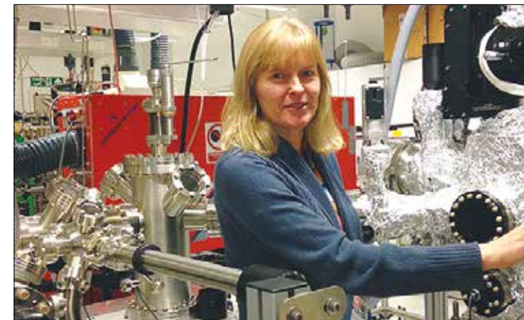
Professor Driscoll in front of an advanced pulsed laser deposition system and a connected X-ray photoelectron spectroscopy system for oxide thin film growth and in-situ analysis
