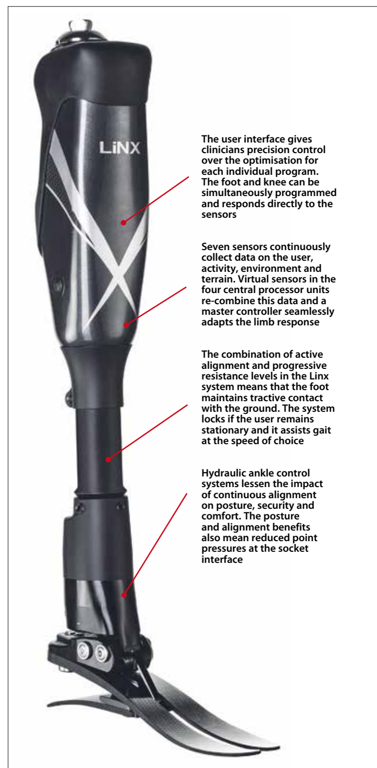
The Linx system fluidly provides physiological motion based on biomimetic principles of gait and posture. The master control unit coordinates the responses of the whole system to achieve smooth interaction between the system parts © Blatchford
