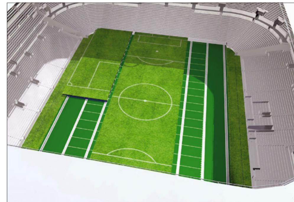
A computer-generated image shows how the three trays carrying the pitch will slide over the artificial NFL field below © Tottenham Hotspur / SCX Special Projects
