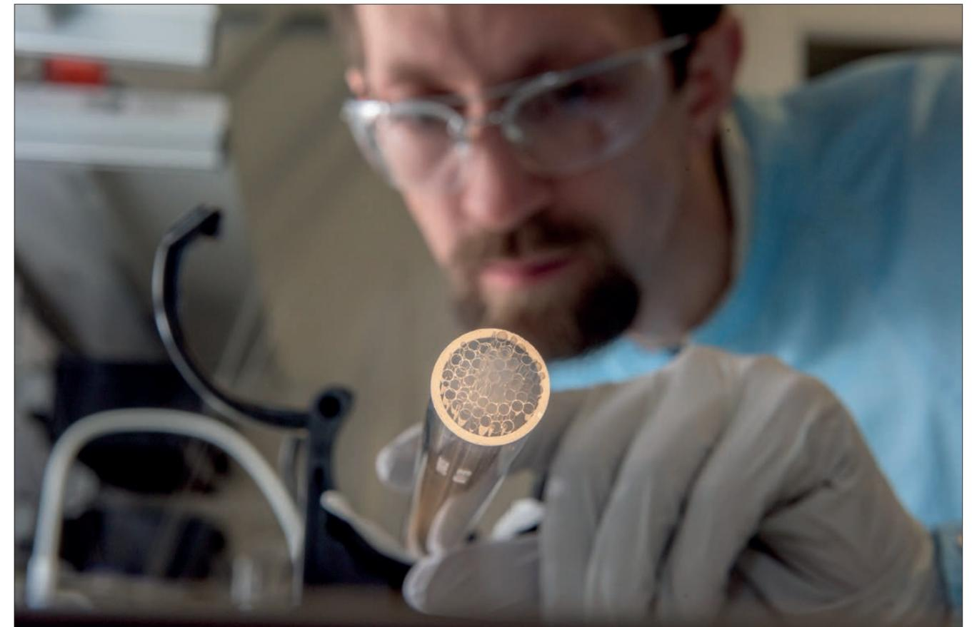
A cane preform being prepared in the Optoelectronics Research Centre lab in the University of Southampton's £120 million cleanroom complex
