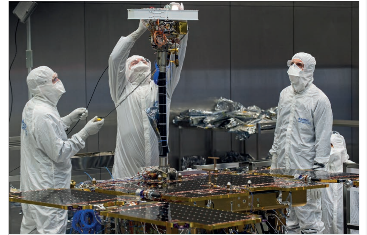
The PanCam being tested on the ExoMars rover in Airbus' cleanroom in Stevenage © Airbus, M. Alexander
