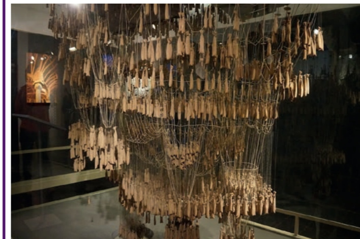
An upside-down force model of the Colònia Güell in the Sagrada Família Museum. Gaudí would hang strings and weights then use the resulting 'catenary curve' to model columns and arches. He would render the model upright by placing a mirror underneath or by taking a photograph © Fundació Junta Constructora del Temple de la Sagrada Família
