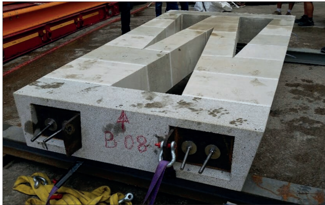
A prototype column, showing the stainless steel rods threaded through the drilled masonry, and the anchorage plates for prestressing © Arup
