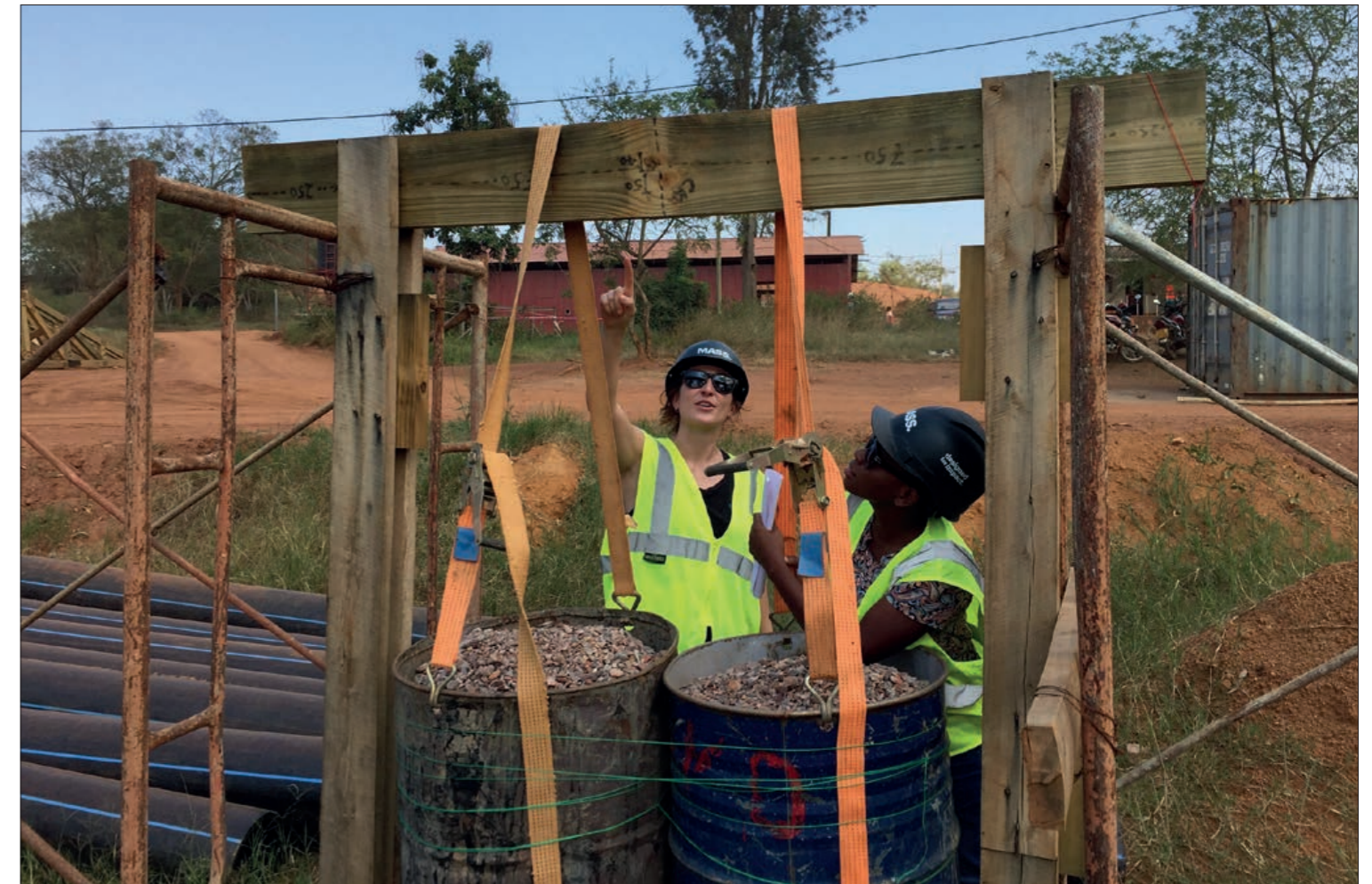
Rosie and Shakira load testing a timber beam with buckets of stone
