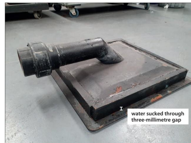
water sucked through three-millimetre gap
