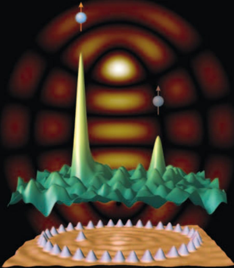
‘Quantum mirage’ formed by an elliptical ‘corral’ of cobalt atoms on a copper surface. (Courtesy of IBM Almaden.)
