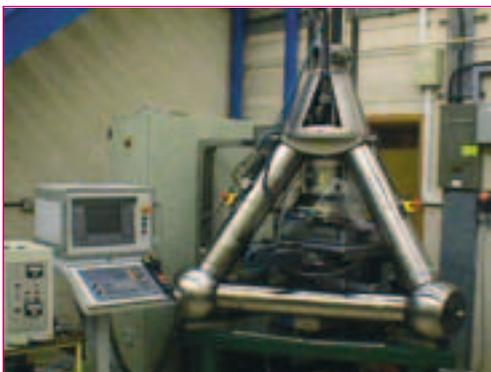
Figure 1: 'Tetraform' ultra-stiff grinding machine.
