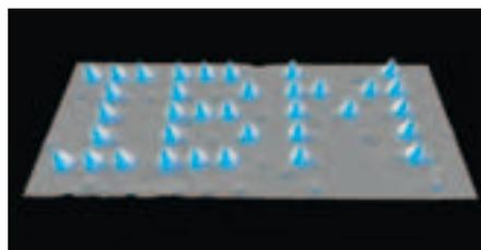
**Figure 5: 35 xenon atoms on a nickel surface spelling out the letters 'IBM'. (Photograph courtesy of IBM.)**
