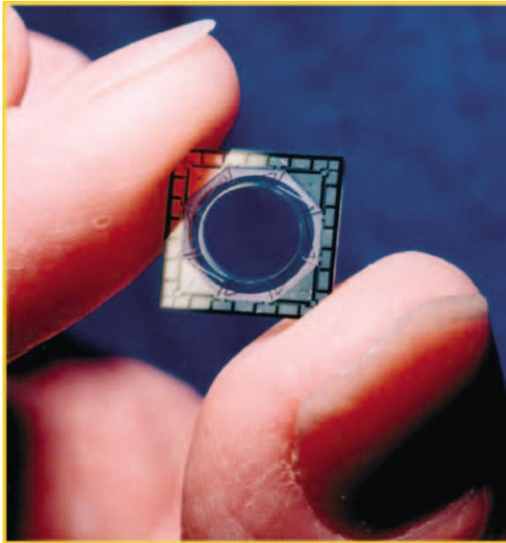
**Figure 3: An example of a practical MEMS device, the BASE rate gyroscope. The ring is about 10 mm across. (Photograph courtesy of BAE SYSTEMS.)**
