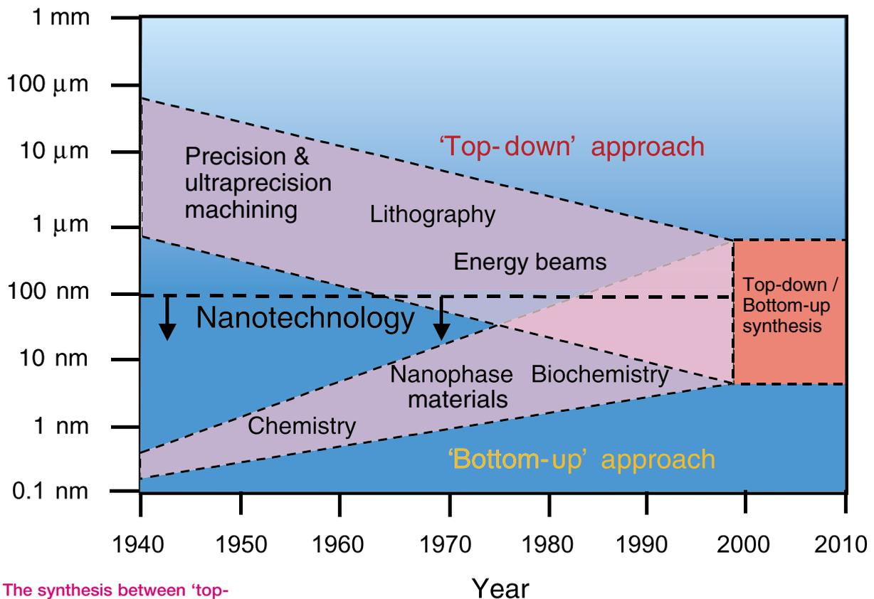
Figure 6: The synthesis between 'top-down' and 'bottom-up' nanotechnology.
