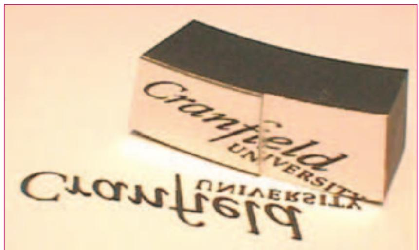
Figure 2: Piece of steel ground using the Tetraform, showing the excellent surface finish that can be achieved.
