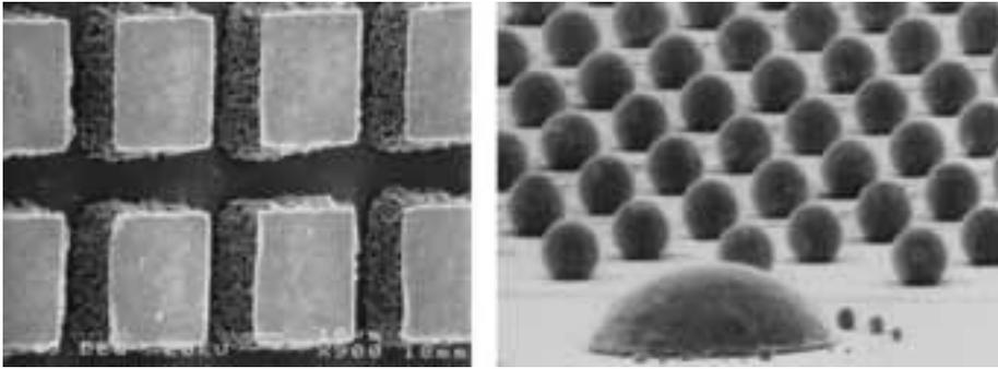
**Figure 4: Uncooled pyroelectric thermal imaging array. The device uses micromachined ceramic elements (left) which are about 30 microns square. These are flip-chip bonded to a silicon readout array using 10 micron diameter bumps of solder (right). (Courtesy of BAE SYSTEMS Infra-red Ltd.)**
