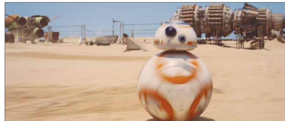
As BB-8 is a round droid that's body moves in all directions while its head stays still, creating the robot proved challenging for the engineers. The ball-bearings on the underside of its head attach it magnetically to the top of the body, which allows it to move freely when the body rotates © Lucasfilm Ltd. & TM. All Rights Reserved
