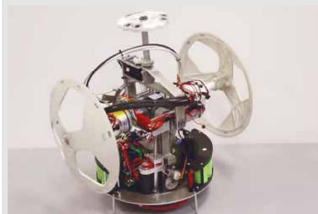
The engineering behind BB-8 was revealed at a *Star Wars* celebration event\* in London in July 2016. This still from a video shown at the event shows the pendulum mechanism inside the robot's body
