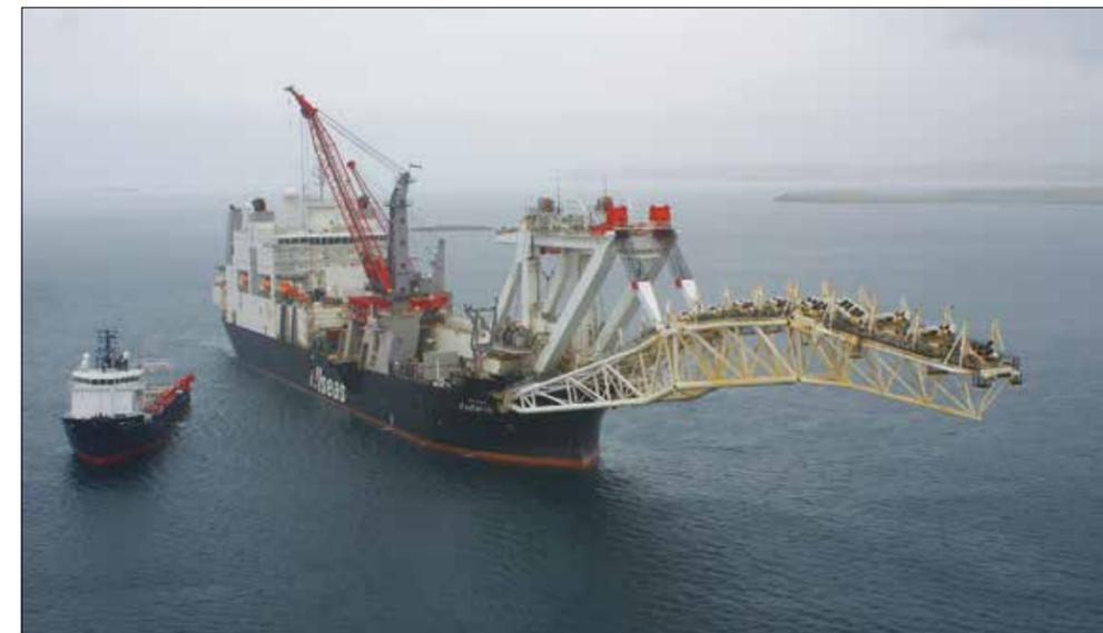
A major part of the Laggan-Tormore project was the offshore installation of two parallel 18-inch flowlines (141 kilometres each) and a 225 kilometre 30-inch export pipeline, all complete with inline valve structures © Total
