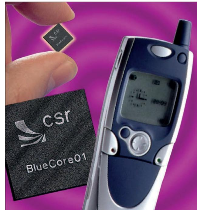
Cambridge Silicon Radio's CSR BlueCore™ chips paved the way for Bluetooth connectivity for several devices
