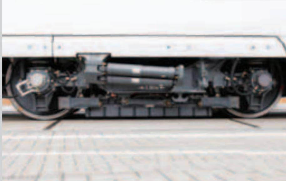
Today, train operators are using Lenz's law to great effect. In Germany's latest ICE3 trains, bogies carry two 1540mm-long magnets with eight coils. In braking, the magnets are lowered to just 7mm above the rail-head. The energised coils induce an opposite magnetic force which acts against the motion of the train, giving a powerful and almost constant deceleration down to 50km/h when conventional brakes take over.
