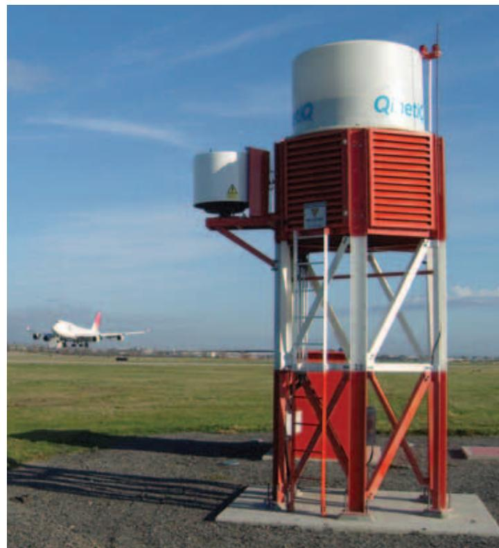
Two to three Tarsier towers continuously scan an airport runway to detect foreign objects and debris © QinetiQ
