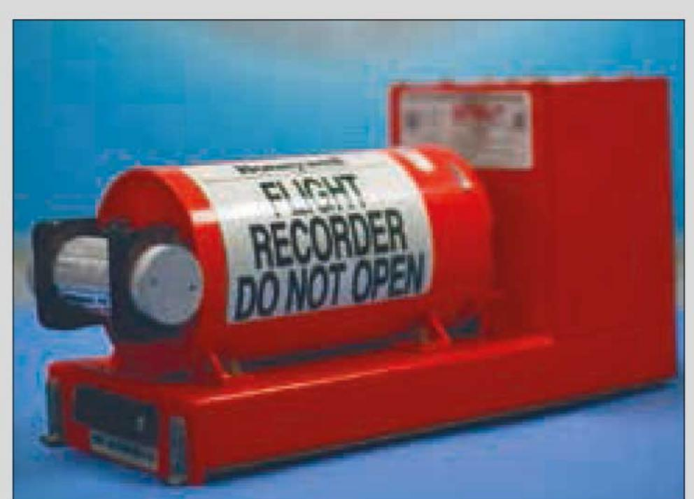
Aircraft accidents are rare, but when they happen can be deadly, sometimes leaving no witnesses. Air accident investigators can use two flight recorders that record four channels of cockpit voice data and hundreds of channels of flight data to find the causes of an accident. These recorders, nicknamed 'black boxes' are actually red or orange and are able to withstand extreme levels of heat and pressure.
