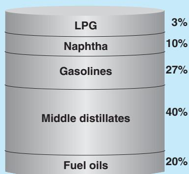
**GTL-FT barrel ( vol%)**
