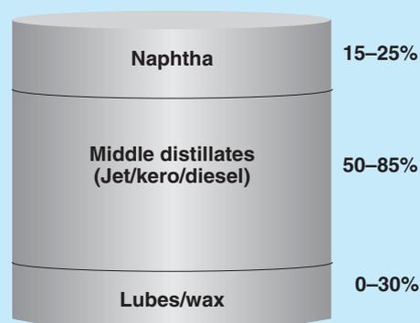
**Figure 2 Comparison of GTL-FT barrel vs conventional barrel**
