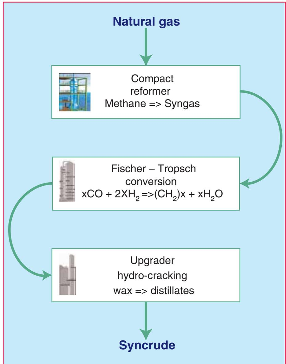
Figure 3 The three major processes involved in converting natural gas into syncrude
