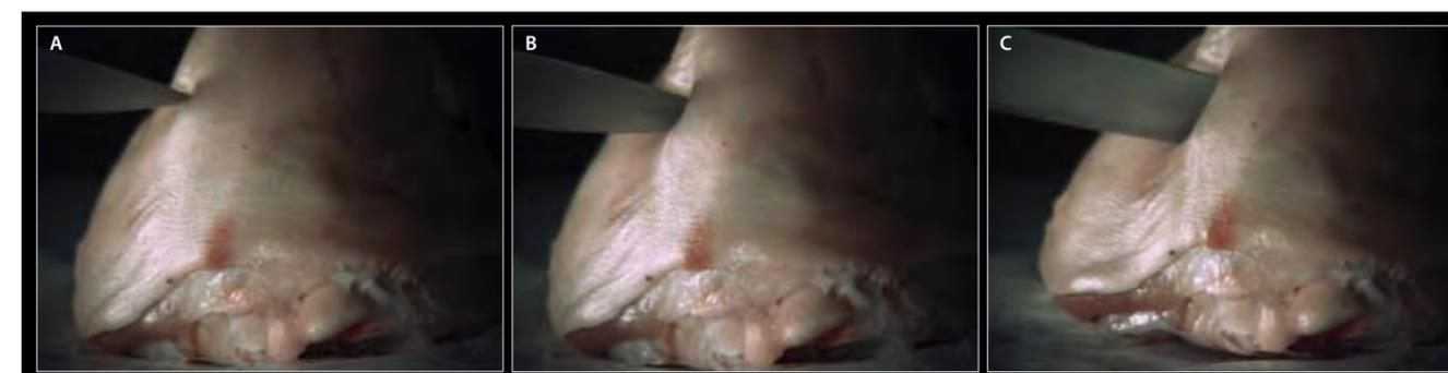
Figure 3: A sequence of images taken from the stabbing test with a sharp Sabatier knife © University of Leicester
