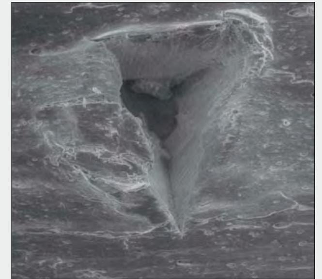
**Figure 6: Environmental scanning electron microscope image of a knife impression in cortical bone** © University of Leicester
