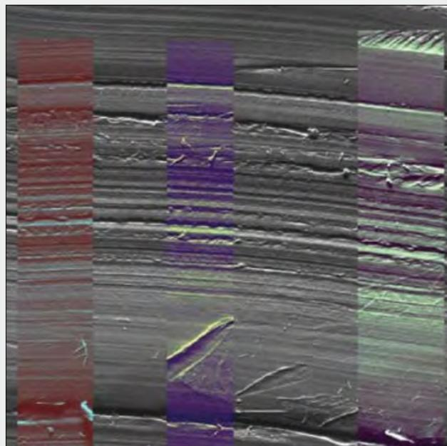
**Figure 5: An environmental scanning electron micrograph image with three inset images showing our ability to match Type C striations. The three inset images (shown by the different colours on the image) are from marks made by the same tool and show the excellent correlation that we are able to achieve between saw marks made with the same tool but different sawyers** © University of Leicester
