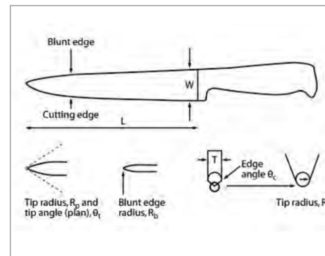
Figure 2: Schematic diagram showing the different parameters to characterise the features of the different knives Figures drawn by Simon Roulstone
