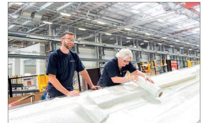
**The assembly of the wind turbine blades at the Hull factory is done entirely by hand, with rolls of fibre shaped to create the composite structure that makes up the blades** © Siemens Gamesa
