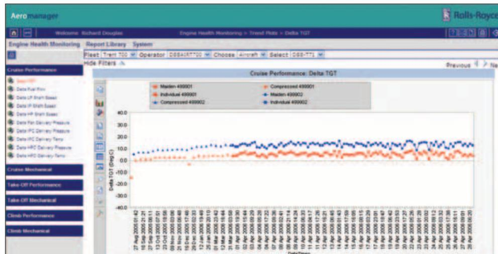
The screen shot shows the corrected Turbine Gas Temperature in cruise – from an Airbus A330. Each data point represents a flight, so this shows two healthy engines with no sudden changes in performance © Rolls-Royce plc
