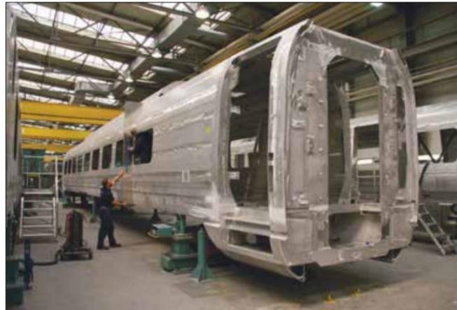
Velaro aluminium car body construction at Siemens in Krefeld, Germany © K Fender
