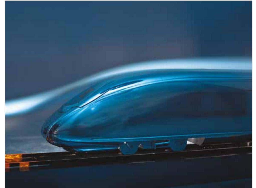
Testing of the aerodynamic behaviour of the Velaro Eurostar in a wind tunnel test. The revision of the aerodynamic concept has led to a reduction in equivalent air resistance surface of approximately 20% compared to earlier designs of Velaro units © Siemens
