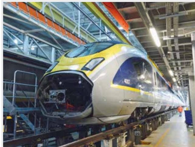
Eurostar's high-security train maintenance depot at Temple Mills in East London was purpose-built for the Class 373 fleet when Eurostar started operating from London St Pancras International station via the completed HS1 high speed rail line in 2007. To accommodate the Class 374, some major changes have been made which reflect how the design of high speed trains has evolved. The vehicles of the new Velaro are built to the European standards for high speed trains and are wider and taller.
