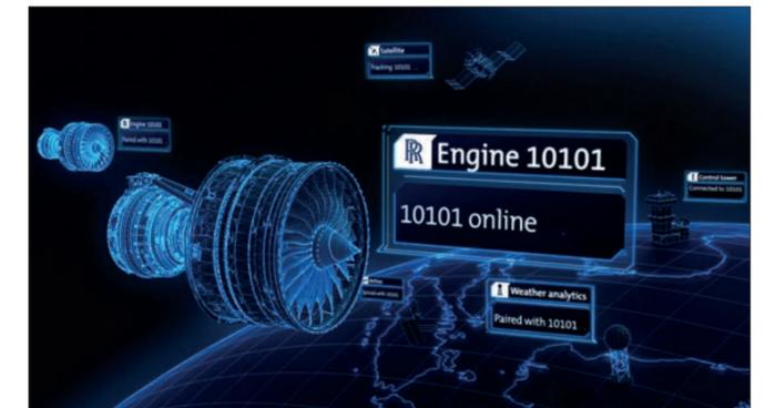
By measuring the engine's condition and ambient environment around it, Rolls-Royce's digital twin enables engineers at the company's operational headquarters in Derby to monitor the condition of an engine in flight, for example between London and Jakarta, with the data relayed back by satellite link, and observe any fluctuations in engine performance that might indicate a component in need of repair or replacement © Rolls-Royce
