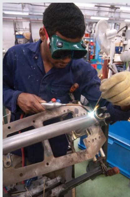
While welding requires temperatures of 1,400° to 1,500°C, brazing is carried out at 950°C, reducing the stresses placed on the metal
