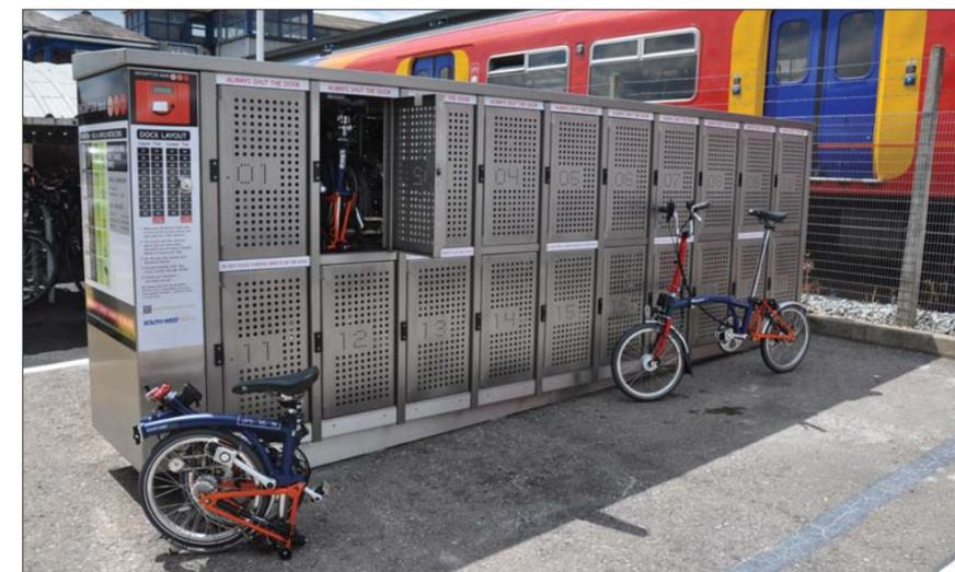
The Brompton Dock in use at Guildford railway station. This unit has capacity for 40 bicycles, 20 on each side
