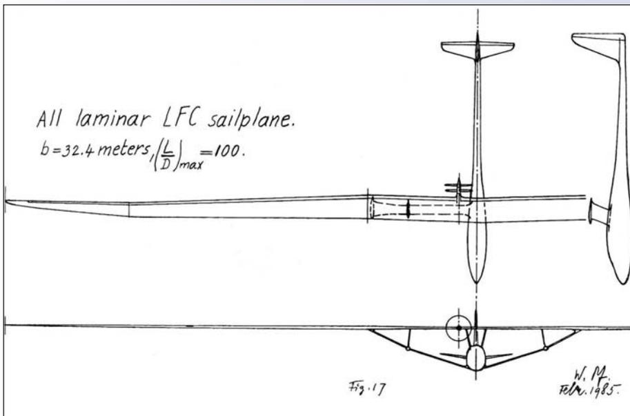
**Figure 6** Pfenninger's 100:1  $L/D$  glider design of 1985
