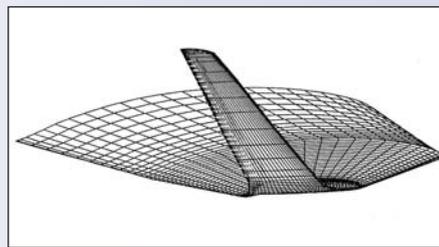
**Figure 7** CFD mesh for a sailplane wing-fuselage winglet junction
