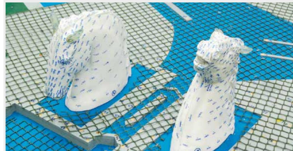
1:100 scale models used for wind tunnel testing © Atkins
