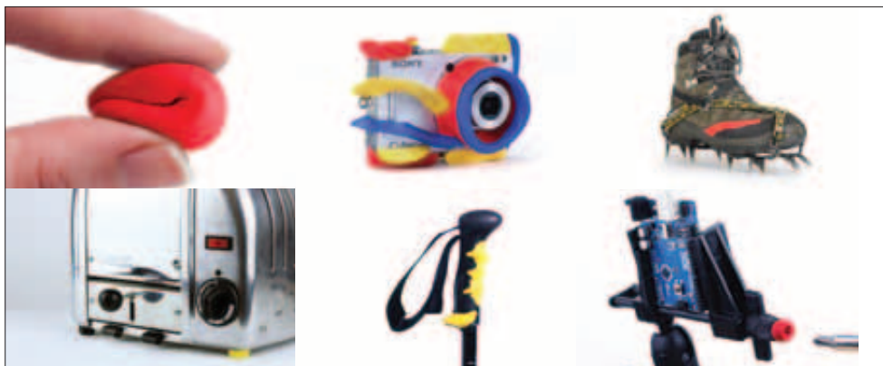
Silicone-based sugru forms a strong bond with aluminium, steel, ceramics, glass, wood and other materials including some plastics such as perspex and rubbers such as silicone and butyl rubber
