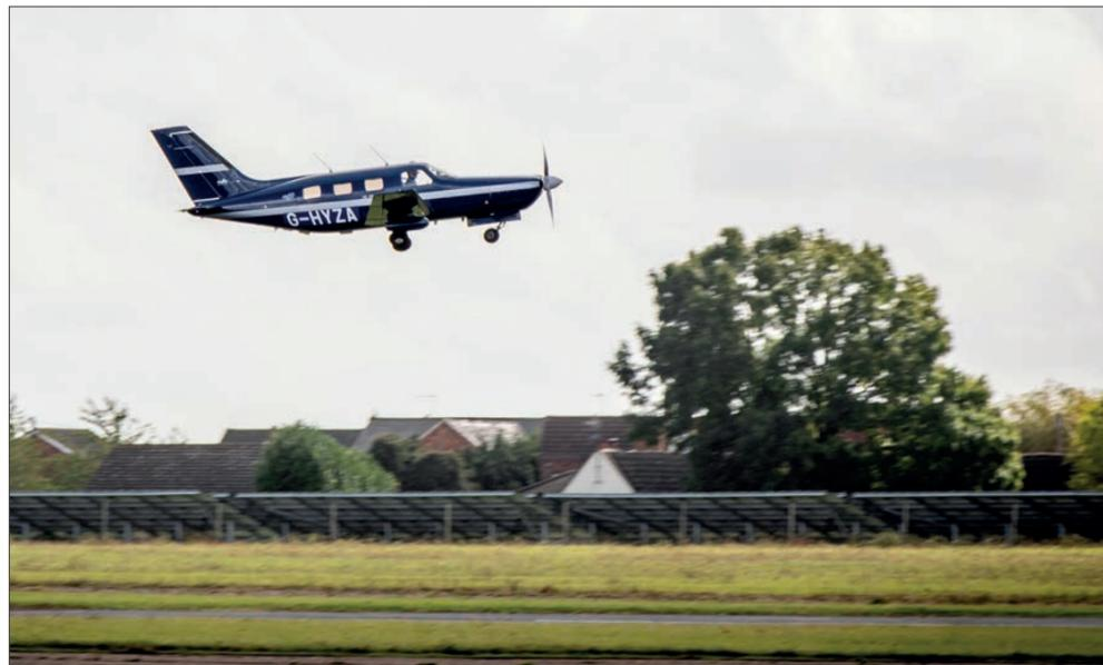
ZeroAvia's six-seater aircraft in flight, powered by the company's hydrogen-electric powertrain
