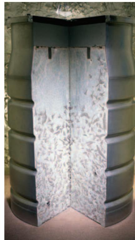
Intermediate level waste is encapsulated in cement in robust stainless steel containers, for long term storage pending disposal. This cutaway shows simulated conditioned ILW in a stainless steel container courtesy Sellafield Ltd
