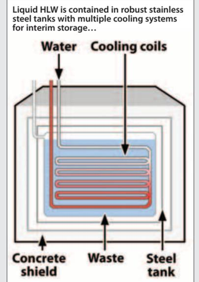
Liquid HLW is contained in robust stainless steel tanks with multiple cooling systems for interim storage...
