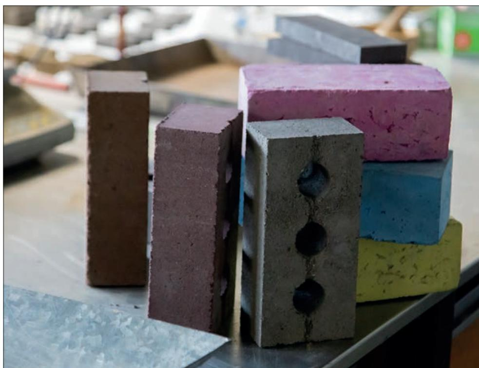
K-briqs can be made in a range of colours by adding recycled pigments to the mix
