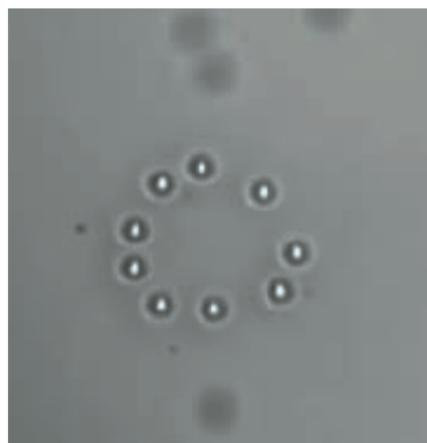
An array of optically trapped beads. Multiple beam traps are commonly created using two different technologies called a spatial light modulator or an acousto-optic deflector. The result is that arrays of many dozens or hundreds of beads may be manipulated in three dimensions simultaneously ©Tomáš Cizmar, University of St Andrews
