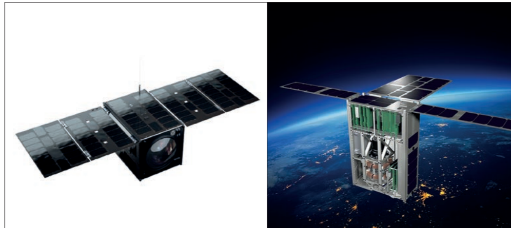
Left: Teledyne e2v's technology is the heart of the 'CASPA-ADM' 12u cubesat (Cold Atom Space Payload – Atmospheric Drag Mission). This will measure tiny variations in atmospheric drag in low Earth orbit, revealing atmospheric density changes useful in climate modelling and orbit decay prediction. It builds on previous miniaturisation and environmental hardening developed in the 6u cubesat CASPA project (right) with partners including the University of Birmingham © image on left courtesy of Clyde Space
