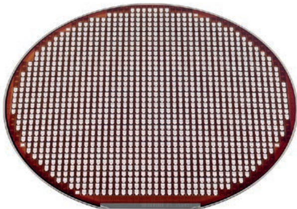
A SiC wafer with MOSFETs, such as those that are paired with diodes and used in the electrical systems of some Formula E racing cars © Infineon Technologies (left), Rohm (right)
