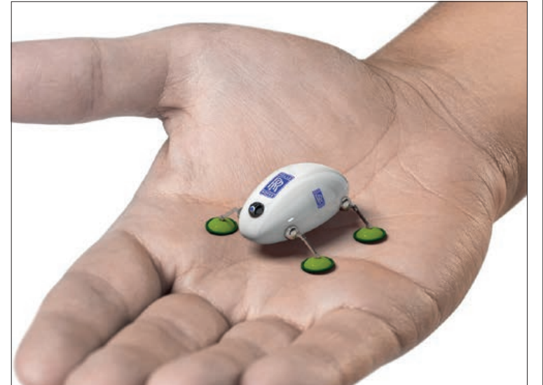
Rolls-Royce has also adopted robot technology in its IntelligentEngine concept for engine maintenance. This combines robotics and digital technologies to speed up inspection and to remove the need to take an engine off an aircraft for maintenance. One concept that Rolls-Royce is working on with researchers from Harvard University and the University of Nottingham is that small ‘swarm’ robots would crawl through an engine to visually inspect hard to reach areas. Another possibility is to permanently embed a network of ‘periscope’ cameras in an engine so that it could inspect itself and report any maintenance requirements © Rolls-Royce
