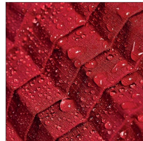
Petit Pli's waterproof material has its structure facing downwards like roof tiles, to ensure no crumbs get stuck, making it the perfect outerwear for children
