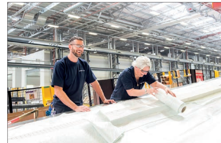
The assembly of the wind turbine blades at the Hull factory is done entirely by hand, with rolls of fibre shaped to create the composite structure that makes up the blades © Siemens Gamesa
