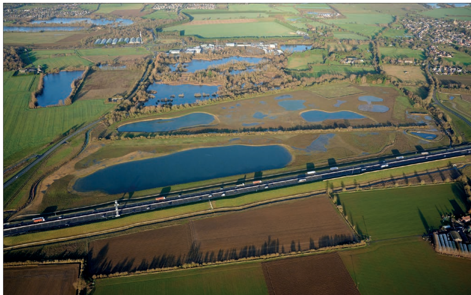
The new A14 Cambridge to Huntingdon road achieved 11.43% biodiversity net gain, largely through converting the borrow pits (which supplied material for embankments) into woodland, grassland, wetland and open water habitat © National Highways
