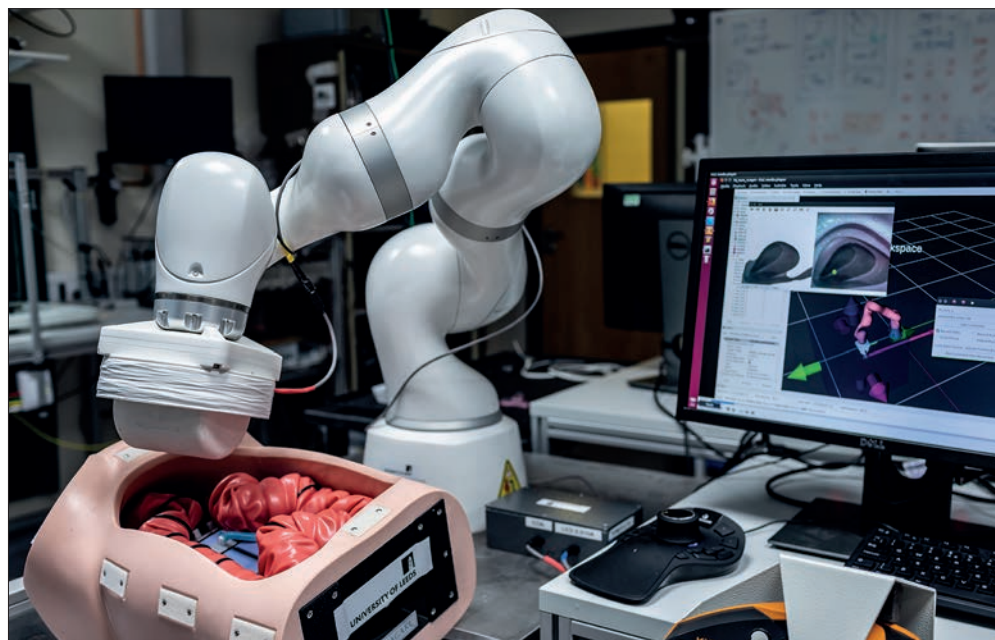
A robotic arm manoeuvres the magnet into place, allowing it to guide the colonoscope through the colon © Mark Webster Photography/University of Leeds
