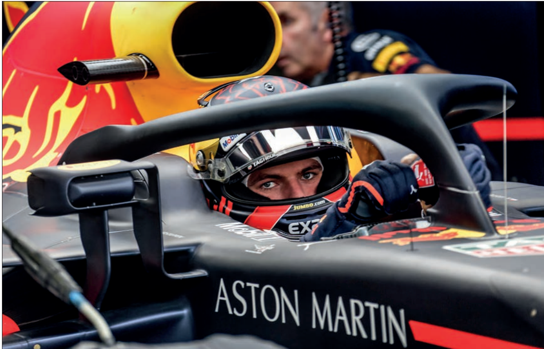
The Halo – the black T-shaped curved structure – is used on vehicles in motorsport racing to protect the driver's head in crashes and from debris © Shutterstock
