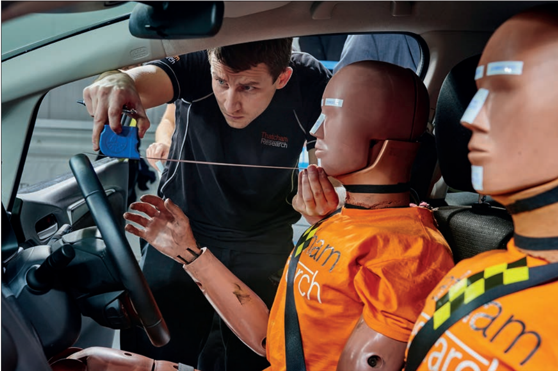
Crash test dummies must be positioned very accurately to ensure that test results are valid © Thatcham Research
