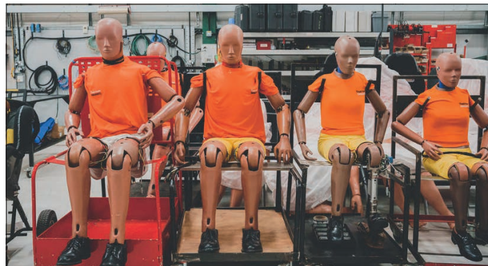
Hybrid-III 50 th percentile male and 5 th percentile female frontal impact crash dummies © Thatcham Research
