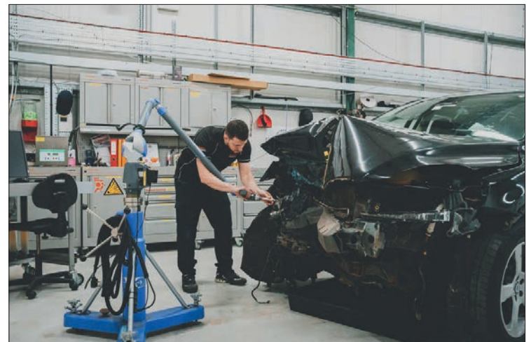
An engineer inspects the damage and takes post-crash measurements © Thatcham Research
