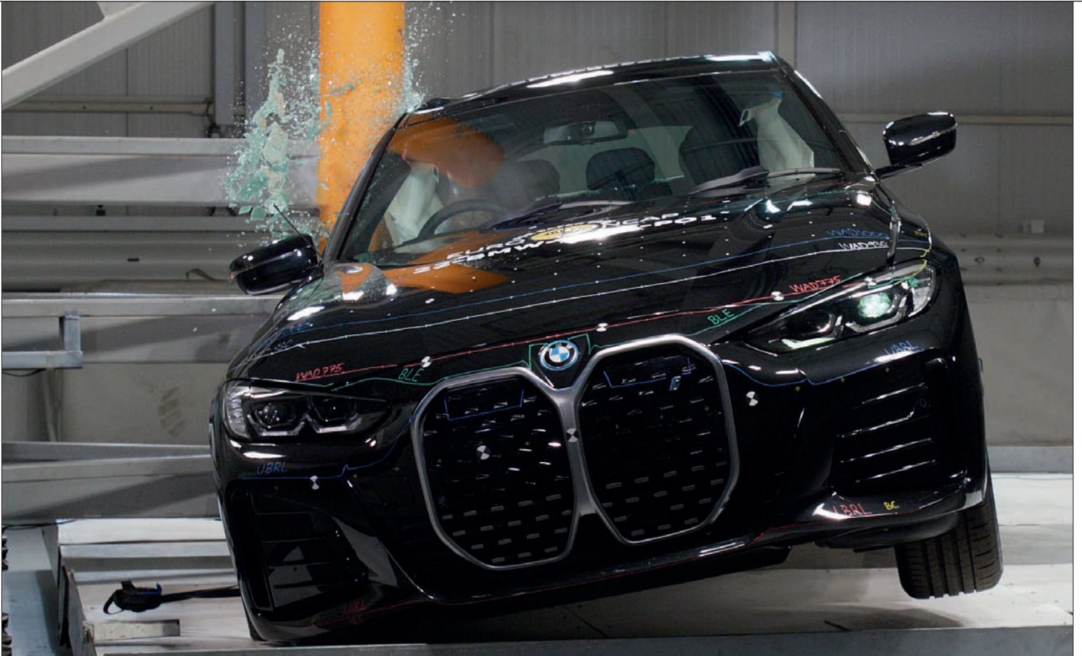
A BMW i4 is subjected to a 32 km/h side pole crash as part of the Euro NCAP test programme © Thatcham Research
